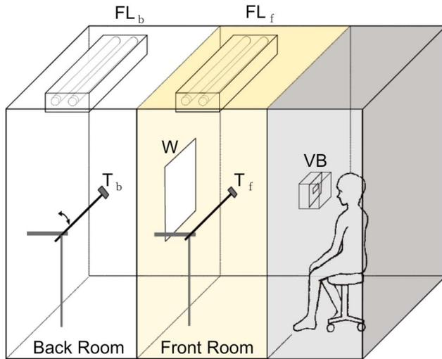
Fig. 1. Scheme of the experimental booth.  $FL_b$ ,  $FL_f$ , lamps in back and front rooms (e.g., white and reddish);  $T_b$ ,  $T_f$ , test patches; VB, viewing box; W, window between back and front rooms.
